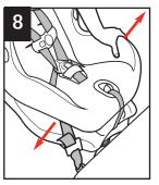
With weakest hand at belt path, tilt and push the child restraint forward and back, and from side to side. If the LATCH belts do not loosen, your child restraint should be secure.
